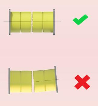
It is recommended from the risk analysis and operation of cellular buffers that they should be replaced every **five years** for safety-relevant applications.
