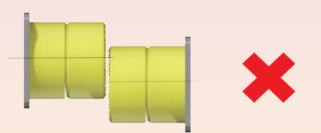
Vertical eccentricity of oppositely mounted buffers must not be higher than 10% of the buffer's diameter.
